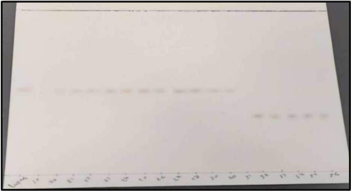
Figure 4. The hexane fraction produced from Combi-flash column chromatography employing hexane: ethyl acetate (8:2) mobile phase was analyzed using thin-layer chromatography. The detection of the compounds in the hexane fraction was done using a 5% H_2SO_4 spray reagent, Subjected to a temperature of 110^\circ C for a duration of 10 minutes.
